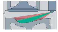
Non-original nozzle element without after treatment  Original MaK nozzle element with after treatment
