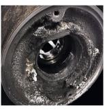
The risk of oil leakage past the piston ring seal is increased. particularly at the turbine end.
