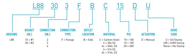
2-part epoxy finish inside and outside for carbon steel housings. Leg assembly. Buna-N butterfly valve package. Carbon steel, 304 SS and 304L SS housings include (2) 304 SS baskets. 300 PSI housings feature slip and blind flange lid assembly. 316/316L housings include (2) 316 SS baskets. Carbon steel not recommended for water use as the epoxy coating is not designed as a corrosion inhibitor.
