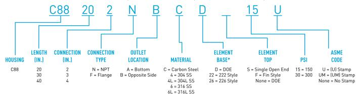
Note: If DOE, it is only required once in the part number and will specify both top and base. Cartridges are not included but the type must be specified when ordering the housing.
