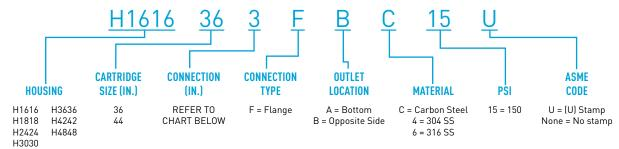
150 psi rating. 2-part epoxy finish on carbon steel housings, exterior only. Buna-N lid seal. Heavy-duty support legs. Removable 2-3/8" heavy wall center guide posts. Bearing assisted davit cover lift closure with swing bolts. Does not include cartridges. Carbon steel not recommended for water use.
