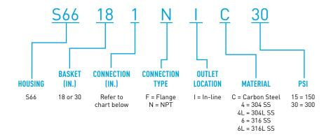
2-part epoxy finish inside and outside for carbon steel strainers. Buna-N lid seal. 3-bolt swing lid. 300 PSI strainers feature slip and blind flange lid assemblies. Carbon steel not recommended for water use as the epoxy coating is not designed as a corrosion inhibitor. Housing cost does not include strainer basket. Strainer baskets must be ordered separately.
