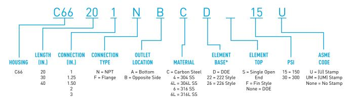
Note: If DOE, it is only required once in the part number and will specify both top and base. Cartridges are not included but the type must be specified when ordering the housing.
