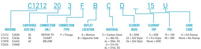
Note: If double open end (DOE), it is only required once in the part number and will specify both top and base. Cartridges are not included but the type must be specified when ordering the housing.
