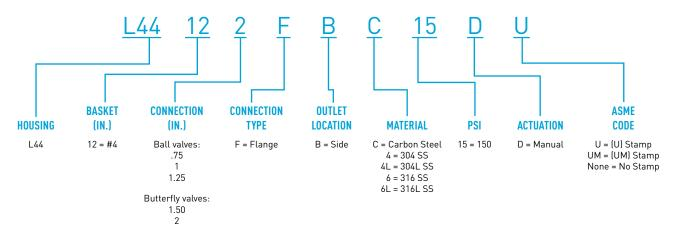
2-part epoxy finish inside and outside for carbon steel housings. 3-bolt swing lid. Buna-N valve package. Leg assembly. Carbon steel, 304 SS and 304L SS housings include (2) 304 SS baskets. 316/316L housings include (2) 316 SS baskets. Carbon steel not recommended for water use as the epoxy coating is not designed as a corrosion inhibitor.
