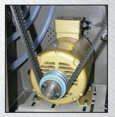
NEMA Premium® efficient inverter-driven motor
