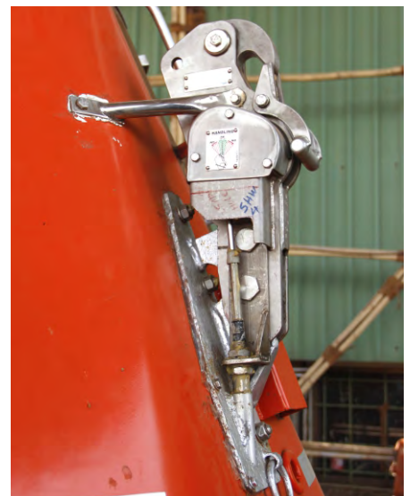
New Hook on SS Foundation
