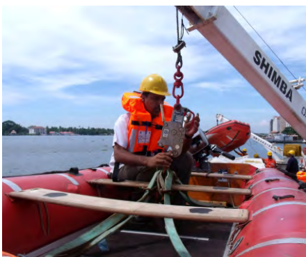
Release Hook Inspection
