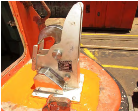
New Hook on FRP Foundation
