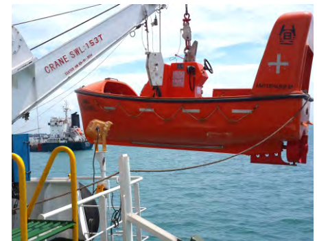
Dynamic Winch Brake Test
