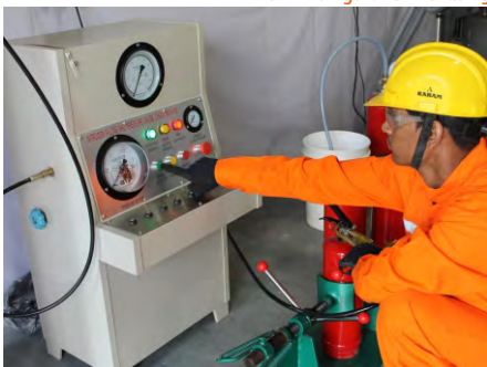
Nitrogen Filling & Gauge Check
