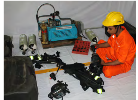
SCBA & EEBD Maintenance and Repair
