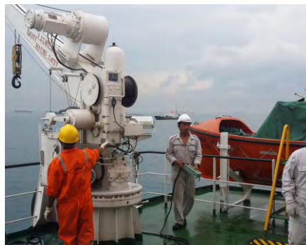
Single Arm Davit Winch Inspection
