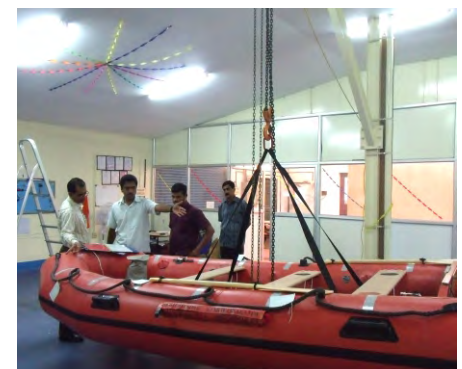
Pressure Test at Service Station
