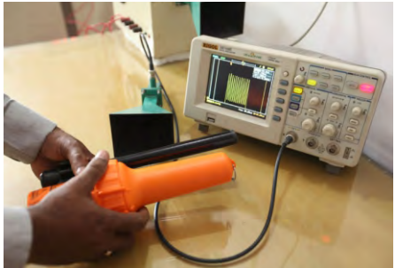
Oscilloscope Reading of Rescue SART
