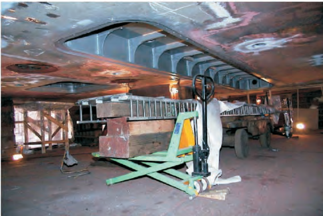
Figure 37 Flush installation blister for the EM 122
