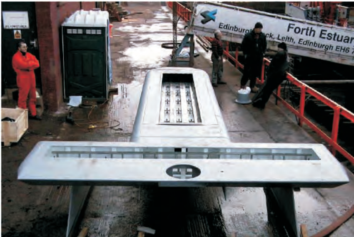
Figure 35 The blister for the EM 122 transducer arrays
