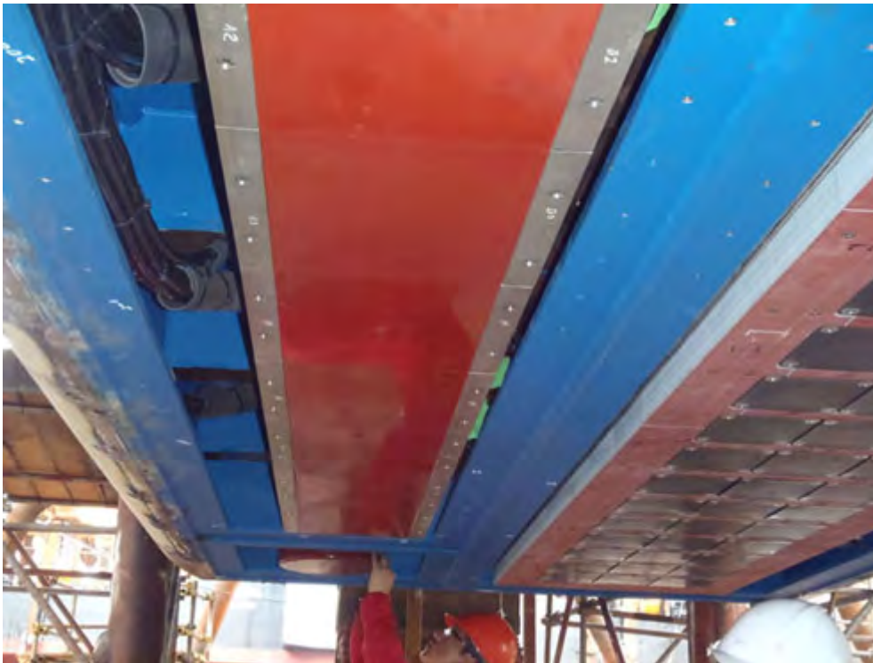
Figure 11 EM 302 Transducer element installation
