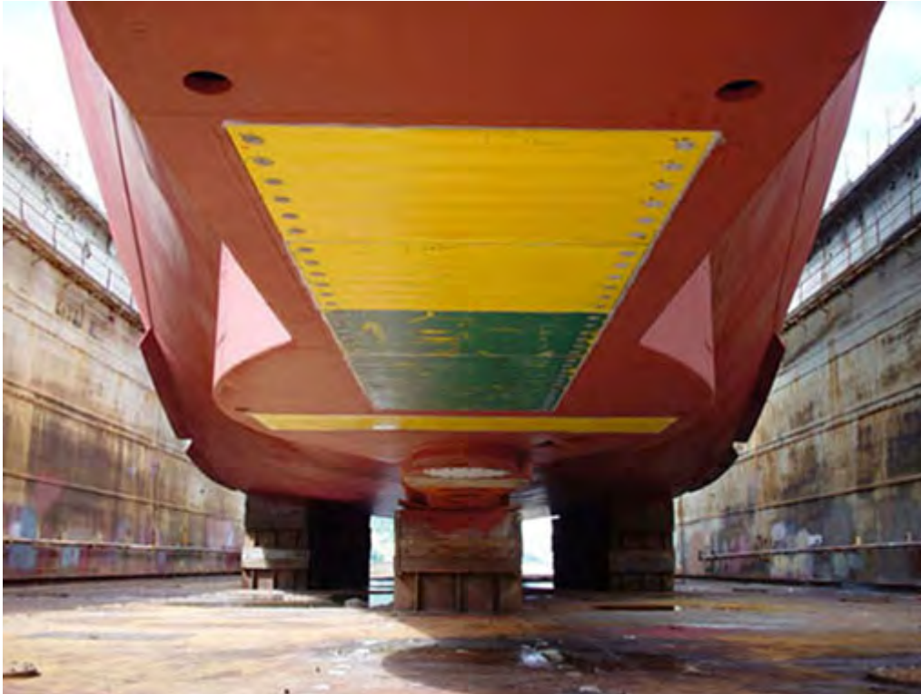
Figure 14 EM 302 Transducer element installation with ice window
