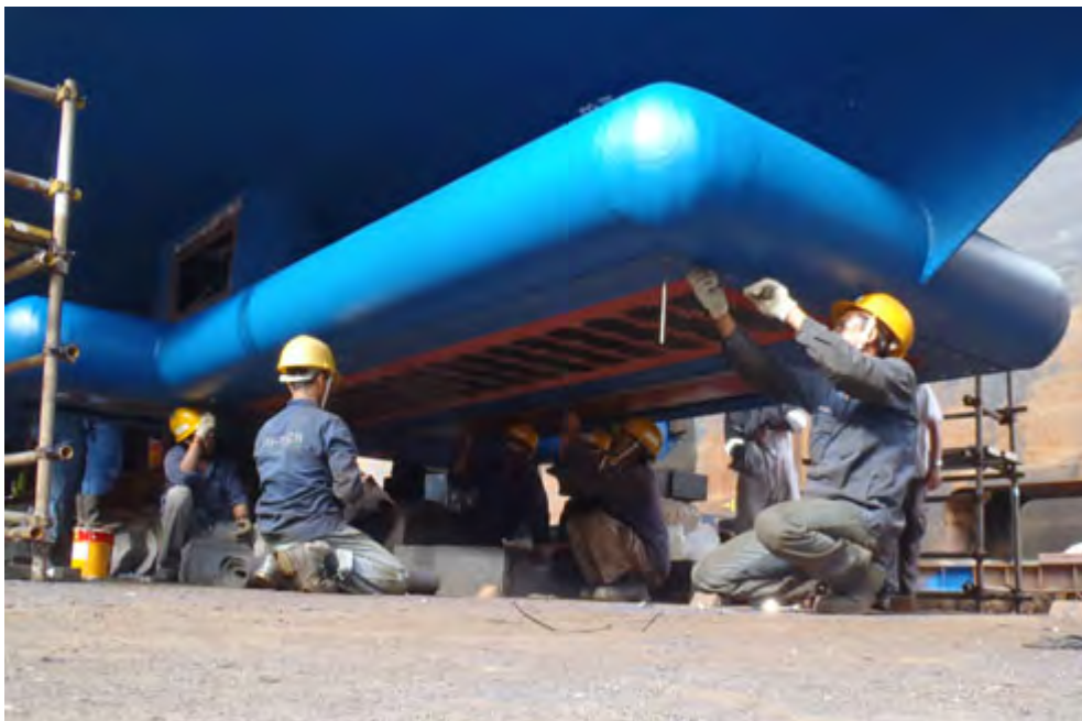
Figure 13 Transducer element installation EM 302
