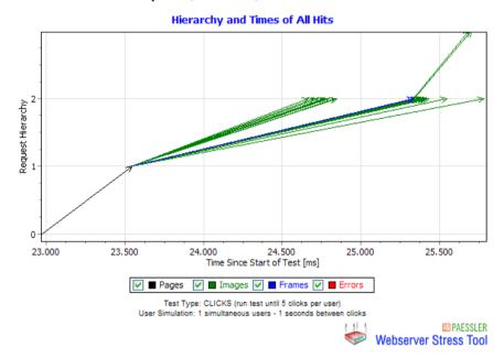
The longer a request took, the further right the arrow ends. As soon as the HTML text of a page request is received, the images are requested from the server and shown in the chart with the green arrows.
