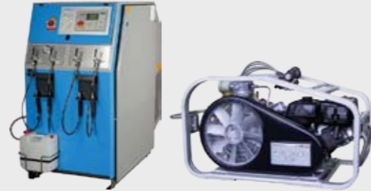
BA Compressor - Electrical and Diesel
